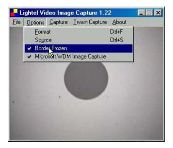
You can unlock the 'Border Frozen' by unchecking this option. With the 'Border Frozen' unchecked, the screen border becomes stretchable and the image can be resized.
