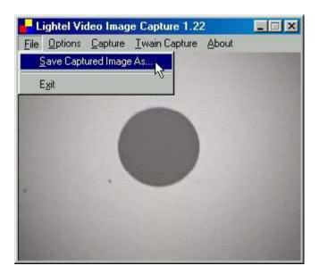
The software provides a default file location at "C:\"and a default base name as "LIC". This means, if you do not specify a file location and a base name, the captured images will be automatically saved as LIC0001, LIC0002, .... under "C:\". You can re-specify the base name and file folder path anytime in your operation:
